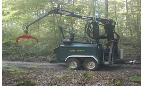
SP 900 - Autonomous SUPER-PAIN 900 chipper, with hydraulic bough-dragger 150 hp motor, On road trailer, double 3.5 t central axles : NOKKA crane 2.5 t/m length of jib 5.10 m
