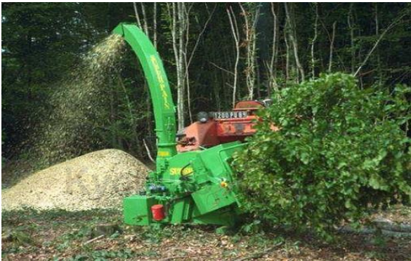
SP 900T on three-points tractor with evacuation neck swinging out 360°
